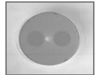
400X magnification for polished PM bare fiber
