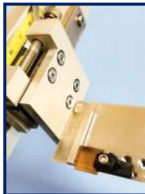
FLeX’s universal carrier supports a variety of component dimensions and does not require wax or holding compounds.
