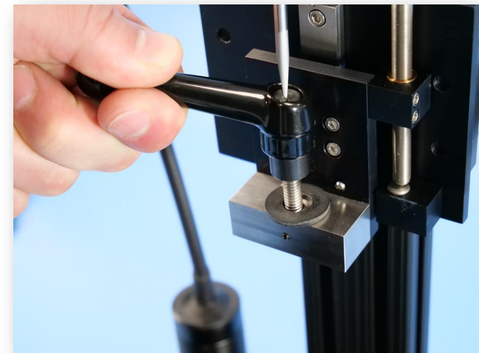
Figure 3. Adjusting Clamping Handle
