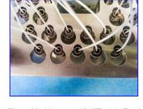
KrellTech's HiCap™ workholders engage with the Scepter Automated Polisher. Adjustable pressure control maintains consistent film contact across the entire connector matrix. An optional water flow system provides easy application of water during the polishing process.
