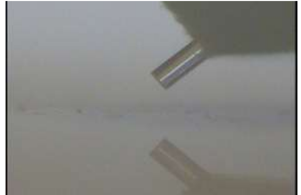
Begin with a cleaved fiber tip.
