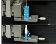
Universal UPC workholders are available that support all connectors/termini with ferrule diameters between 1.25 to 3.2mm.
